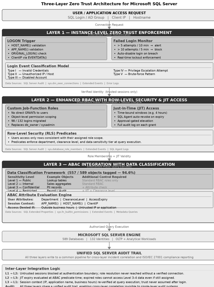
Figure 1. Three-Layer Zero Trust Enforcement Pipeline for Microsoft SQL Server. The diagram illustrates the sequential enforcement pipeline spanning authentication (Layer 1), authorization and session lifecycle (Layer 2), and query execution (Layer 3), with inter-layer integration logic and a unified audit trail.
